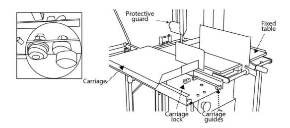
To remove the carriage, the car lock should be moved 90° from its own axis counterclockwise, as shown in the figure.
