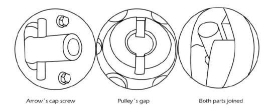
To avoid pulleys from coming off from the arrow while functioning, lock it as shown in the example figures. The following operation is made without tension on the band saw blade.
