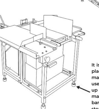
It is recommended to place the band saw machine on the floor, use the leveling legs up to 3 inches to make sure the cutting band saw machine is steady and secure.
