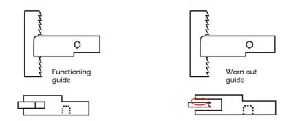
The tugsten guides allow the machine to control the movements the band saw blade has while operating, the guides have normal wear. The following figures shows when the guides has worn and should be replaced.
