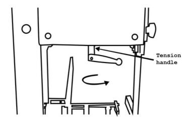
This equipment incorporates a total tension system (automatic), whichs allows the band saw blade reach the adequate tension and the pulleys and guides to align. This system is designed to maximize the meat saw machine potential and help the operator have better cuts, less waste and prolong the saw blade's life. Apply food grade grease in the screw cap included in the machine.
